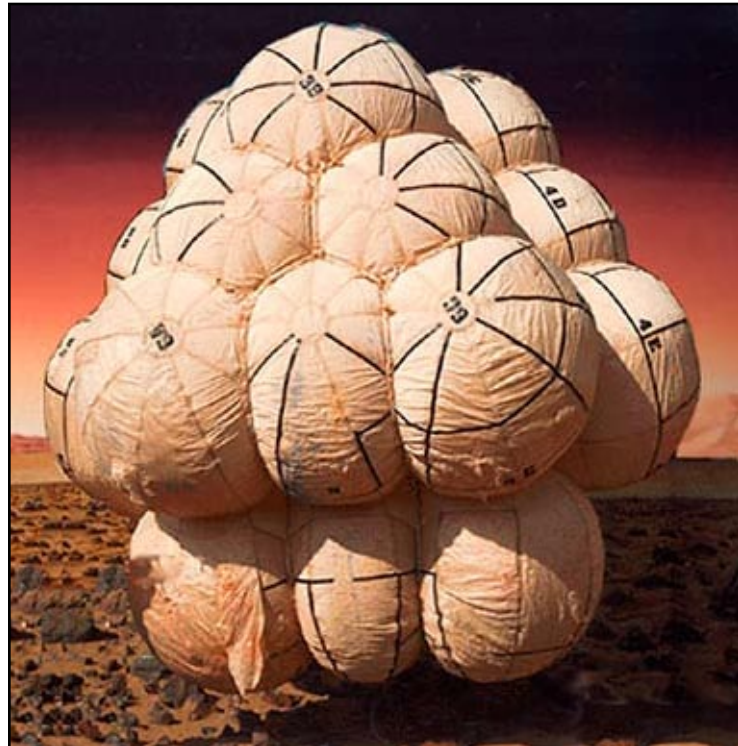
Mars air bags made with fabric manufactured by Warwick Mills
